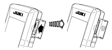
② After completion of setting of the card, close the smart media cover. By closing the cover, it is possible to perform communication.
