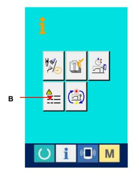
Error record of the sewing machine you use is displayed in the error record screen, and you can check the error.
