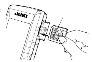
① The smart media card stops once in the protruding state by approximately 10 mm while inserting the card. Further, apply force to insert the card and ease up the force when it is reached to the end. Setting is completed when the card has returned by approximately 1 mm.
