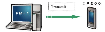
Connect the personal computer with IP200 and transmit data to the sewing machine after creation of data with PM-1. When IP200 becomes the data input screen, automatically the trial sewing screen is displayed. For the operating procedure of PM-1, see HELP of PM-1 or the like.
